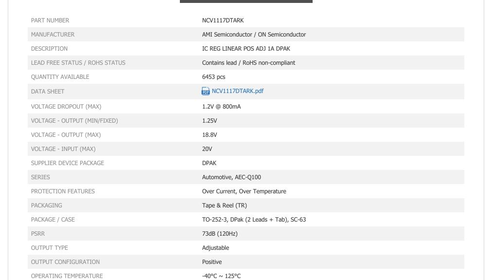
Linear Voltage Regulator IC Positive Adjustable 1 Output 1.25 V  $\sim$  18.8 V 1A DPAK DETAILED DESCRIPTION 10mA CURRENT - QUIESCENT (IQ) **CURRENT - OUTPUT** 1A
