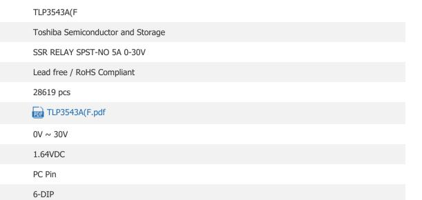
**SERIES** TLP3543A **PACKAGING** Tube 6-DIP (0.300", 7.62mm) PACKAGE / CASE
