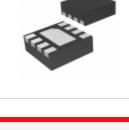
Manufacturers: AMI Semiconductor / ON Semiconductor Description: DCDC BUCK CONVERTER
