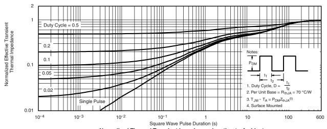
Normalized Thermal Transient Impedance, Junction-to-Ambient
