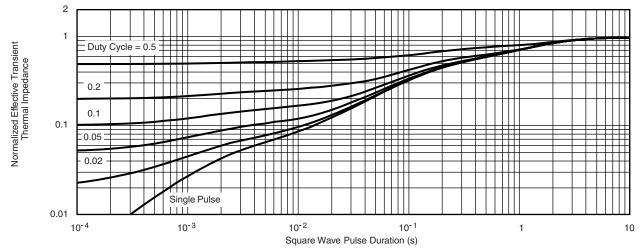
Normalized Thermal Transient Impedance, Junction-to-Foot
