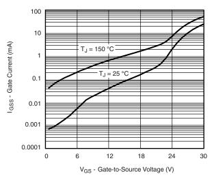
Gate Current vs. Gate-Source Voltage
