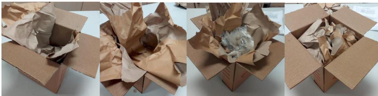
Figure 2: 'Paper Void Fill' encapsulating the bags of contacts inside the Carton.
