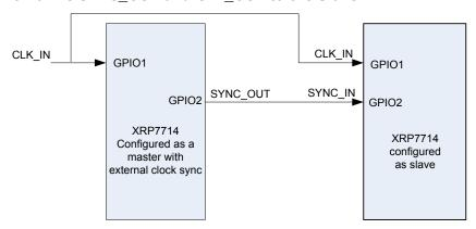
Fig. 29: External Clock Synchronization Master Slave Combination
