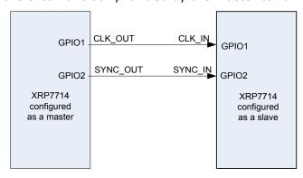
Fig. 28: Master/Slave Configuration of the XRP7714
