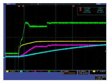
Fig. 22: VCCA (green) Startup Waveform
