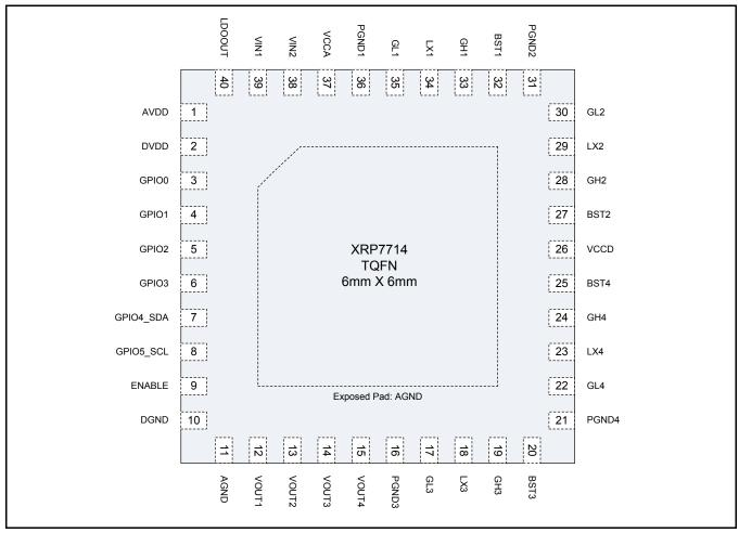
Fig. 3: XRP7714 Pin Assignment
