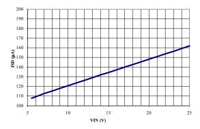
Fig. 10: Shutdown Current 5.1V to 25V
