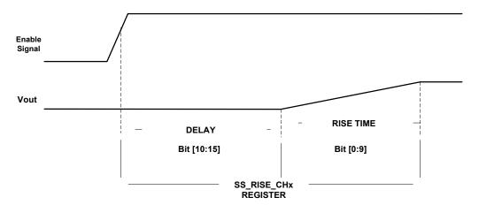
Fig. 24: Channel Power Up Sequence
