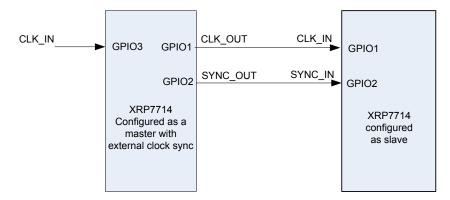
Fig. 30:Alternative External clock synchronization Master Slave combination
