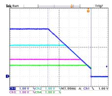
Fig. 15: Sequential Soft-stop V<sub>OUT</sub> Shutdown=0.8V, 3A load CH1:3.3V, CH2:5V, CH3:1V, CH4:1.8V
