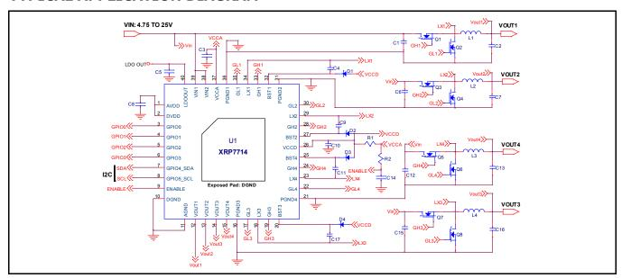
Fig. 1: XRP7714 Application Diagram
