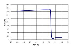
Fig. 11: Shutdown Current 4.8V to 5.1V
