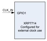
Fig. 27:XRP7714 Configured For External Clock Use
