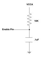
Fig. 21: RC Delay for Enable taken from VCCA
