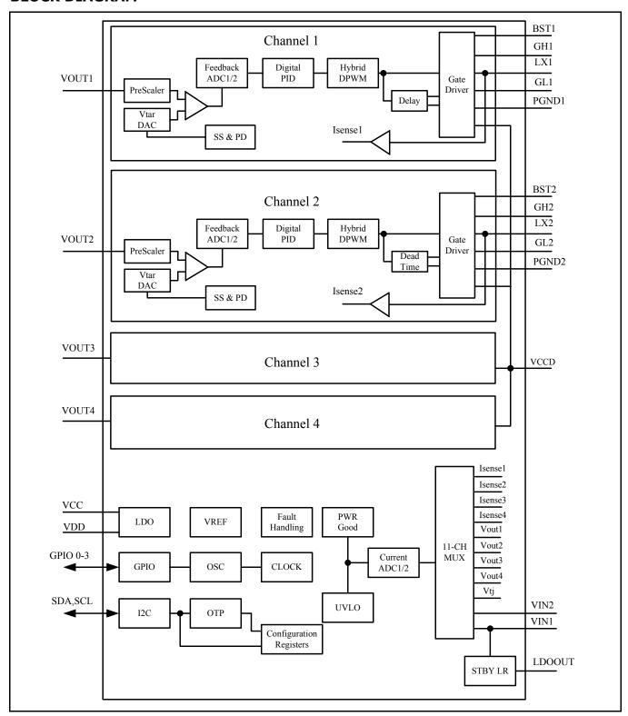
Fig. 2: XRP7714 Block Diagram
