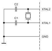
The Oscillator can operate in three different modes, each optimized for a specific frequency range. The operating mode is selected by CKSEL3..1 fuses or by CSEL3..1 field as shown in Table 5-9.
