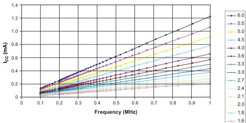
Figure 5-115. Active Supply Current versus Low Frequency (0.1 - 1.0MHz)
