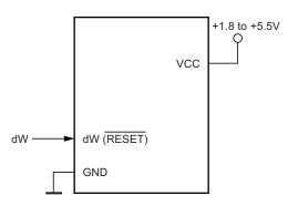
Figure 5-95 shows the schematic of a target MCU, with debugWIRE enabled, and the emulator connector. The system clock is not affected by debugWIRE and will always be the clock source selected by the CKSEL Fuses.
