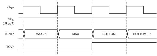
Figure 5-38 shows the same timing data, but with the prescaler enabled.
