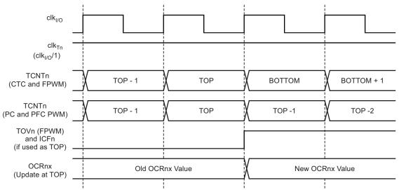
Figure 5-57 shows the same timing data, but with the prescaler enabled.
