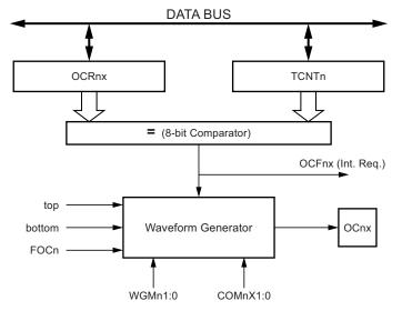
The OCR0A Register is double buffered when using any of the Pulse Width Modulation (PWM) modes. For the Normal and Clear Timer on Compare (CTC) modes of operation, the double buffering is disabled. The double buffering synchronizes the update of the OCR0A Compare Register to either top or bottom of the counting sequence. The synchronization prevents the occurrence of odd-length, non-symmetrical PWM pulses, thereby making the output glitch-free.
