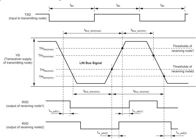
Figure 4-23. Definition of Bus Timing Characteristics
