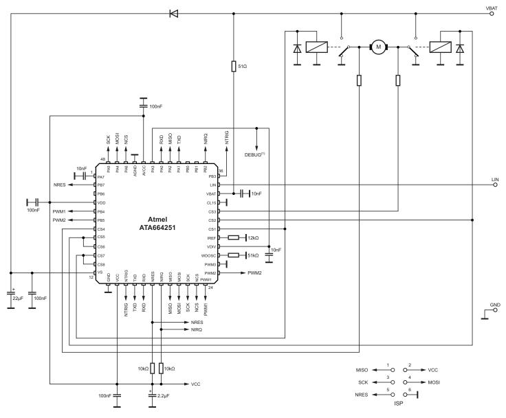
(1) Note: If the Watchdog shall be disabled directly after power-up (e.g. for microcontroller programming or debugging purposes) the pin VDIV must be tied to High Level until the Reset phase ends (Positive slope at pin NRES).
