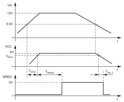
Figure 4-19. VCC Voltage Regulator: Ramp-up and Undervoltage Detection
