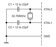
12 to 22pF capacitors may be necessary if parasitic impedance (pads, wires and PCB) is very low.
