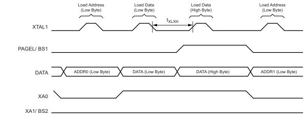
Note: 1. The timing requirements shown in Figure 5-109 (i.e.,  $t_{DVXH}$ ,  $t_{XHXL}$ , and  $t_{XLDX}$ ) also apply to loading operation.
