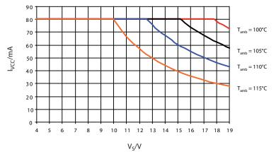
Because the VCC voltage generation is usually fundamental to system operation, there is a thermal prewarning implemented. The thermal monitor of the VCC output transistor can indicate a critical temperature condition of  $T_{VCCprew}$  by means of an interrupt and the status bit OTVCC in the status register of the chip. The microcontroller can thus react to these events by shutting down external loads that use the VCC or reducing its own power consumption in order to avoid a thermal shutdown.
