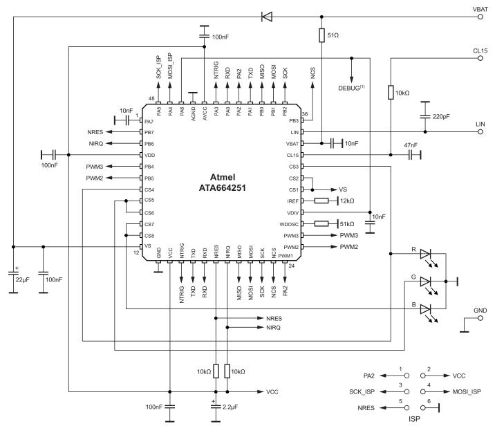
(1) Note: If the Watchdog shall be disabled directly after power-up (e.g. for microcontroller programming or debugging purposes) the pin VDIV must be tied to High Level until the Reset phase ends (Positive slope at pin NRES).
