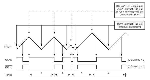
The Timer/Counter Overflow Flag (TOV1) is set each time the counter reaches BOTTOM. When either OCR1A or ICR1 is used for defining the TOP value, the OC1A or ICF1 flag is set accordingly at the same timer clock cycle as the OCR1A/B Registers are updated with the double buffer value (at TOP). The interrupt flags can be used to generate an interrupt each time the counter reaches the TOP or BOTTOM value.
