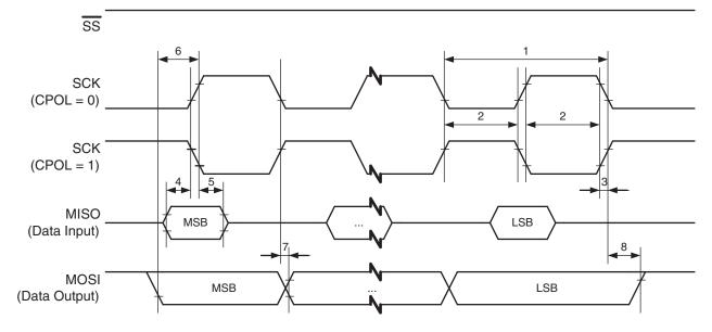
Figure 5-113. SPI Interface Timing Requirements (Slave Mode)
