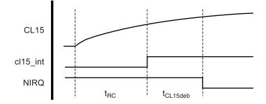
In the diagram above, the voltage at the CL15 pin is shown. Due to the R/C filter, the voltage does not immediately increase but instead slowly over time. As soon as the voltage exceeds approximately 3V, the internal debouncing time t<sub>CL15deb</sub> starts. After this elapses, a wake-up is indicated by a falling edge on the NIRQ pin.
