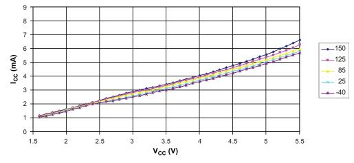
Figure 5-118. Active Supply Current versus V<sub>CC</sub> (Internal RC Oscillator, 128kHz)
