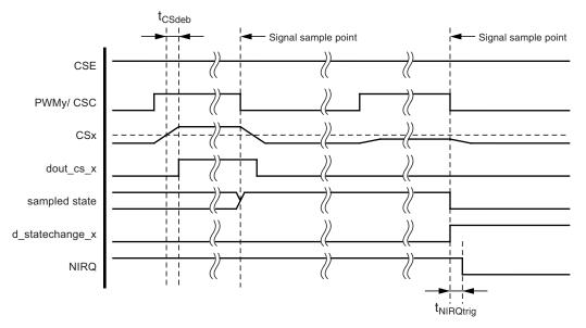
The output state of the HV comparator is sampled with each falling edge of the PWMy or CSC signal. As soon as the sampled state changes, an interrupt request is given.
