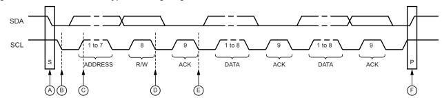
Referring to the timing diagram (Figure 5-66 on page 175), a bus transfer involves the following steps:
