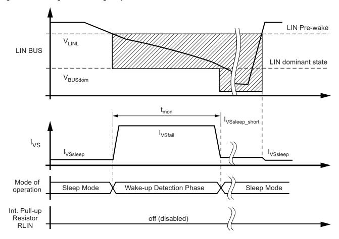
Figure 4-7. Floating LIN Bus During Sleep Mode
