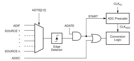
Using the ADC Interrupt Flag as a trigger source makes the ADC start a new conversion as soon as the ongoing conversion has finished. The ADC then operates in Free Running mode, constantly sampling and updating the ADC Data Register. The first conversion must be started by writing a logical one to the ADSC bit in ADCSRA register. In this mode the ADC will perform successive conversions independently of whether the ADC Interrupt Flag, ADIF is cleared or not.
