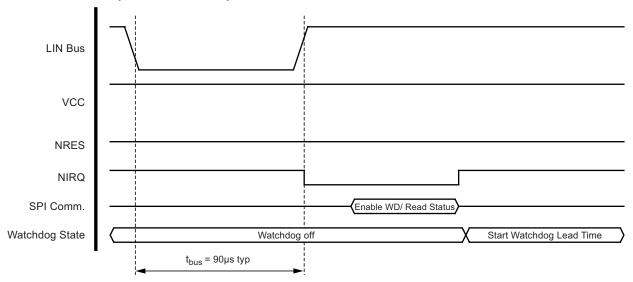
The negative edge on the NIRQ pin indicates a change of conditions, in this case a wake-up request at the LIN bus. The microcontroller can check the IRQ source by assessing the "IRQS1" and "IRQS0" bits in the status register. Note that if a watchdog operation is desired, it must be enabled via the configuration register.
