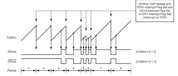
The Timer/Counter Overflow Flag (TOV1) is set each time the counter reaches TOP. In addition the OC1A or ICF1 flag is set at the same timer clock cycle as TOV1 is set when either OCR1A or ICR1 is used for defining the TOP value. If one of the interrupts are enabled, the interrupt handler routine can be used for updating the TOP and compare values.
