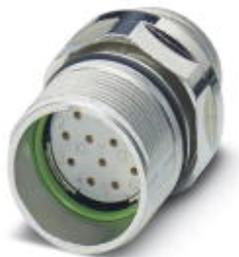
Device connector for front wall, straight, shielded: yes, SPEEDCON locking, M23, No. of pos.: 12, type of contact: Socket, Solder connection, Axial seal, Central fastening M20 x 1.5, can be positioned via a locking nut
