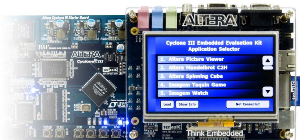
Figure 5. View of the Application Selector User Interface
