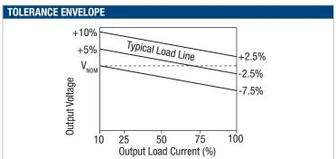
The voltage tolerance envelope shows typical load regulation characteristics for this product series. The tolerance envelope is the maximum output voltage variation due to changes in output loading.
