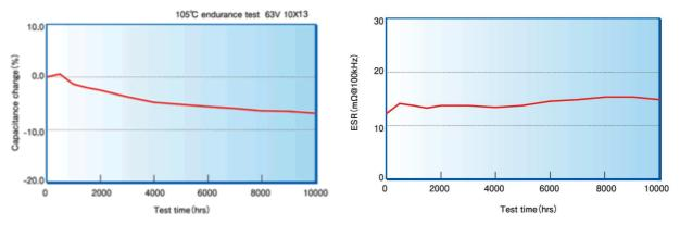
Graph-1: High temperature load test result of PZA Series(Capacitance change/ESR)
