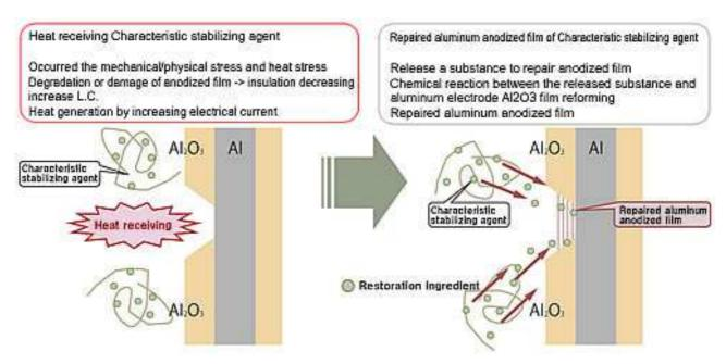
Fig-2 Aluminum anaolized film repair (Image) by characteristic stabilizing agent
