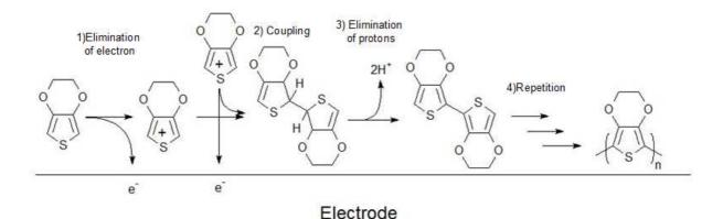
Fig-1 PEDOT Polymerization process
