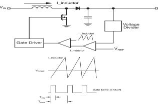
Figure 3. SKIP Mode Waveform
