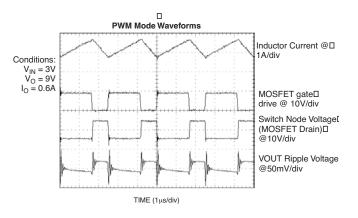
Figure 5 - PWM mode waveforms
