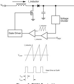
Figure 6: PWM Control Loop
