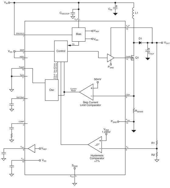
Figure 2. MIC2186 SKIP Mode Block Diagram
