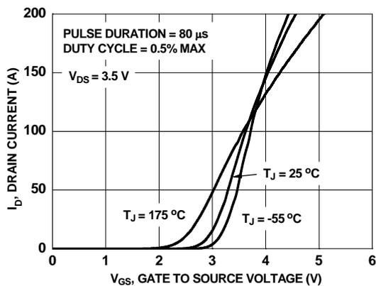
**Figure 5. Transfer Characteristics**
