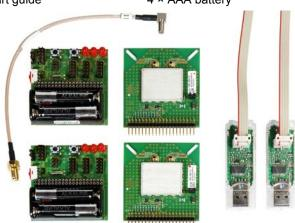
From left to right: MS-147 to SMA cable, 2 × CBB, 2 × REB, 2 × USB level converter.
