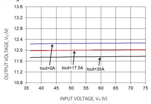
Figure 8. Typical Output Voltage Regulation vs. Output Current.
