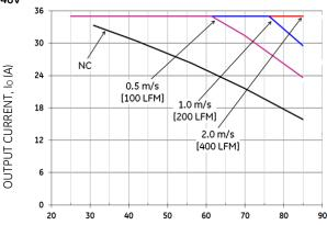
LOCAL AMBIENT TEMPERATURE, Ta (°C) Figure 21. Output Current Derating for the Base plate QSVW035A0B-H with 0.5" heatsink in the Transverse Orientation; Airflow Direction from Vin(-) to Vin(+); Vin = 48V
