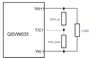
Figure 15. Circuit Configuration to Trim Output Voltage.
