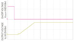
Figure 5. Typical Start-Up Using Vin with Remote On/Off enabled, negative logic version shown.
