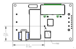
Figure 16. Location of the thermal reference temperature TH.
