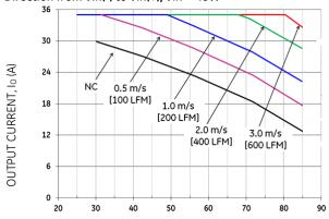
LOCAL AMBIENT TEMPERATURE,  $T_A$  (°C) Figure 19. Output Current Derating for the Base plate QSVW035A0B-H in the Transverse Orientation; Airflow Direction from Vin(-) to Vin(+); Vin = 48V.
