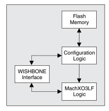
The MachXO3LF must be in user mode in order to access the WISHBONE interface. Accessing and updating the resources made available by the configuration logic must be done in Transparent mode. Attempting accesses to the configuration logic in offline mode causes a deadlock because the MachXO3LF leaves user mode.
