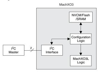
There are two hardened I<sup>2</sup>C controllers in a MachXO3L/LF device, a primary and a secondary. The primary controller provides an interface to the MachXO3L/LF Configuration Logic. The primary I<sup>2</sup>C controller is the only one that permits access to the Configuration Logic OR can be a User Mode I<sup>2</sup>C controller. The Secondary I<sup>2</sup>C controller is always a User Mode I<sup>2</sup>C controller.
