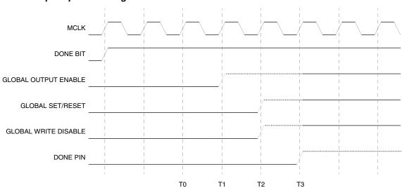
Figure 18. Wake-up Sequence Using Internal Clock
