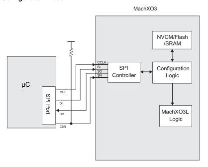
The SSPI port is active when the MachXO3L/LF is in Feature Row HW Default Mode state. Diamond's default preference for the SLAVE\_SPI\_PORT is to ENABLE the port. Use the Spreadsheet View to DISABLE the SLAVE\_SPI\_PORT preference in your design to keep the SSPI port to be used as general purpose I/O in user mode. Lattice recommends you keep a secondary programming port active in the event the SSPI port is accidentally disabled.
