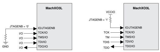
It is critical when using the JTAGENB feature that logic attached to the JTAG I/O pins not contend with a JTAG programming system. The external logic must ignore any JTAG transactions performed by an external programming system.
