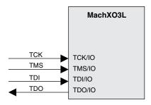
The JTAG port can become general purpose I/O. By setting the JTAG\_PORT preference in the Diamond Spread-sheet View to the DISABLE state. When the JTAG port is in the DISABLE state the JTAGENB pin becomes a dedicated input. Driving the JTAGENB low disables the JTAG port and the four JTAG pins become general purpose I/Os. Driving the JTAGENB input high enables the JTAG port. Figure 9 shows JTAG port behavior under the control of the JTAGENB.
