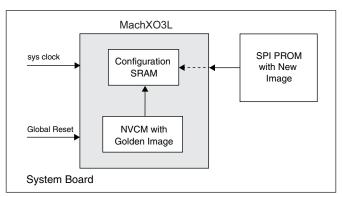
The example assumes that you have the golden image stored in NVCM in order to initiate the system, and will then use SPI PROM as a resource for image updates without disturbing the system. Figure 16 shows the process flow for performing this task.
