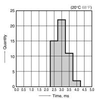
6. Functional shock resistance Tested sample: AEJ11012, 3 pcs. Half-wave pulse of sine wave: 11 ms Detection time: 10µs. Applied direction: 6 directions Applied cycle: Each of 3 cycles
