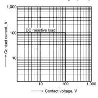
2. Carrying current limit Connection electric wire: 40mm<sup>2</sup> Ambient temperature: 85°C 185°F
