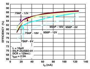
FIGURE 3. EFFICIENCY, L = 10 $\mu$ H WITH DCR = 129m $\Omega$ , Co = 4x4.7 $\mu$ F/50V
