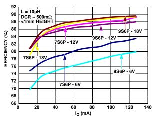
FIGURE 4. 3 EFFICIENCY, L = 10 $\mu$ H WITH DCR = 500m $\Omega$ , 1mm, C<sub>O</sub> = 4x4.7 $\mu$ F/50V
