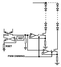
FIGURE 17. SIMPLIFIED CURRENT SOURCE CIRCUIT
