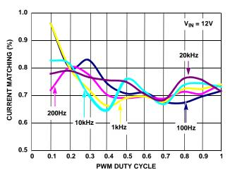
FIGURE 7. CURRENT MATCHING vs DUTY CYCLE vs DIMMING FREQUENCY
