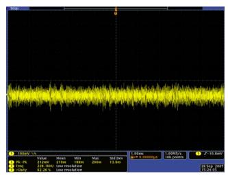
FIGURE 15. RIPPLE VOLTAGE (54 LEDs,  $V_{IN}$  = 12V, 20mA EACH,  $C_{OUT}$  = 4x4.7 $\mu$ F/50V)
