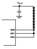
FIGURE 19. GROUPING MULTIPLE CHANNELS FOR HIGH CURRENT APPLICATIONS
