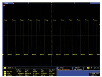
FIGURE 14. LX ZOOM IN AT 50% DIMMING (54 LEDs, 20mA,  $V_{\text{IN}}$  = 12V)
