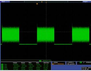
FIGURE 10. I<sub>L</sub> AT 50% PWM DIMMING (54LEDs, 20mA,  $V_{IN}$  = 12V, L = 8.2 $\mu$ H)
