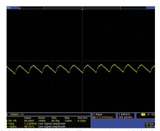
FIGURE 16. RIPPLE VOLTAGE ZOOM IN (54 LEDs,  $V_{\text{IN}}$  = 12V, 20mA EACH,  $C_{\text{OUT}}$  = 4x4.7 $\mu$ F/50V)
