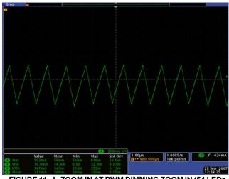
FIGURE 11. I<sub>L</sub> ZOOM IN AT PWM DIMMING ZOOM IN (54 LEDs, 20mA,  $V_{IN}$  = 12V, L = 8.2 $\mu$ H)
