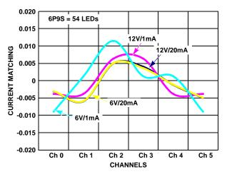
FIGURE 6. CHANNEL-TO-CHANNEL CURRENT MATCHING
