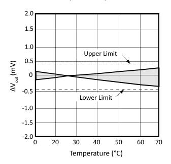
Figure 3: V<sub>OUT</sub> vs. Temperature (VRE310J)
