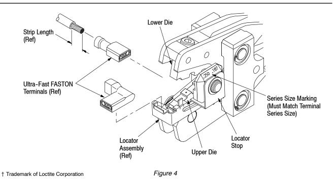
6. Activate tool to complete the crimp. Open the jaws by squeezing the adapter rollers together; then remove the crimped terminal.
