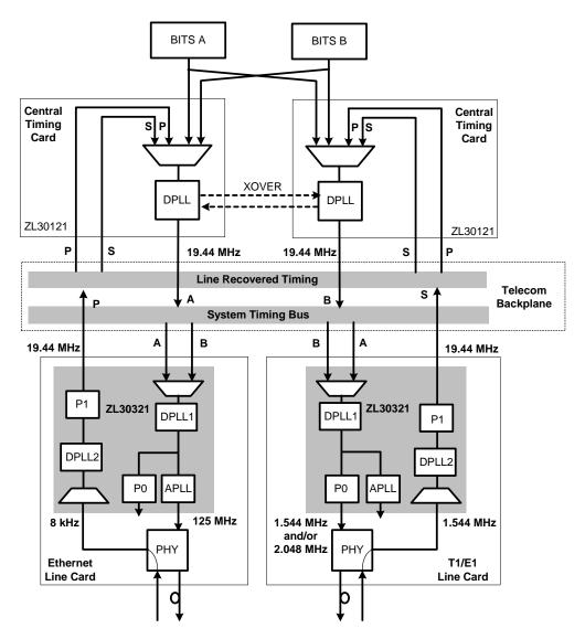
Figure 2 - Typical Application of the ZL30321
