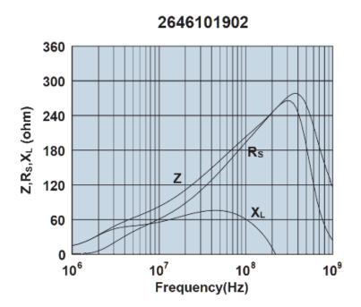
Impedance, reactance, and resistance vs. frequency.
