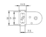
A simple winding handle can be made using a laser cut sheet and an M3 nut and bolt. The drawing to the right shows suitable dimensions The following technical drawings of the built PCB and motor should help you to design your enclosure and winding handle. All dimensions are in mm
