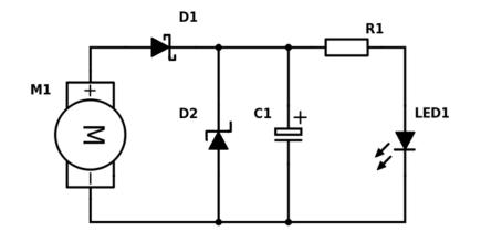
The circuit diagram for the Windup Torch is shown above. It is a very simple circuit. The motor (M1), acting as a generator, powers the circuit when turning the handle. The faster rotation of the generator the higher the voltage supplied to the circuit
