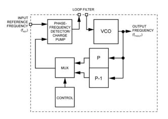
Figure 1. Fractional-N Synthesizer Architecture
