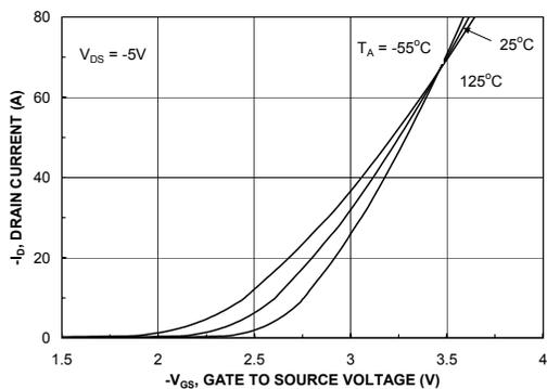
Figure 5. Transfer Characteristics.
