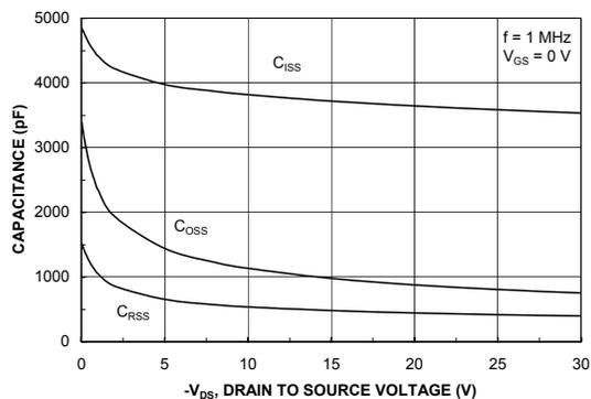
Figure 8. Capacitance Characteristics.
