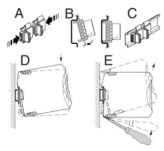
Figure 6 Mounting and removing
