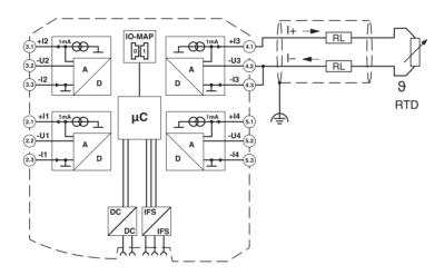
Figure 8 2-wire connection technology
