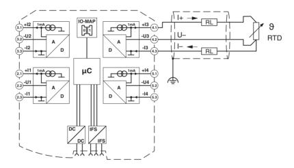
Figure 9 3-wire connection method
