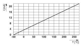
Figure 5 Current strength [mA] depending on the temperature [°C]
