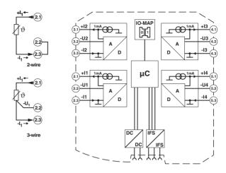
Figure 2 RAD-PT100-4-IFS basic circuit diagram
