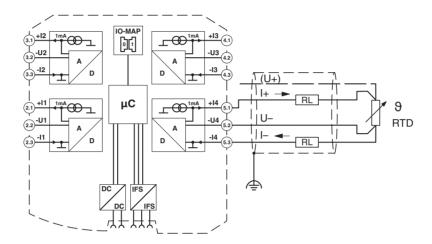
Figure 10 4-wire connection technology
