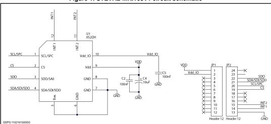
Figure 1: STEVAL-MKI168V1 circuit schematic
