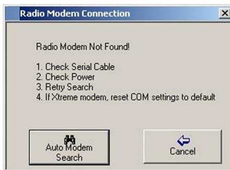
Figure 3. Radio Modem Not Found Screen
