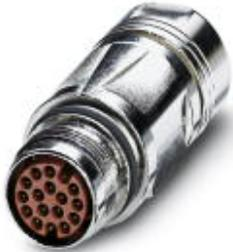
Coupler connector, straight, SPEEDCON locking, M17, Number of positions: 8, Type of contact: Male connector, Crimp connection, shielded: yes, Cable diameter: 10 mm...12.5 mm
