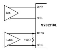
Figure 2d. Driving BEN with LVDS Outputs
