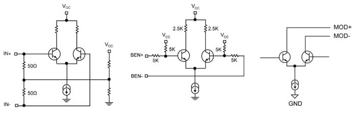
Figure 1a. Simplified Input Stage
