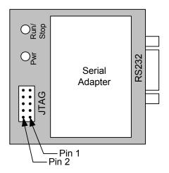
Figure 5. Serial Adapter JTAG Connector
