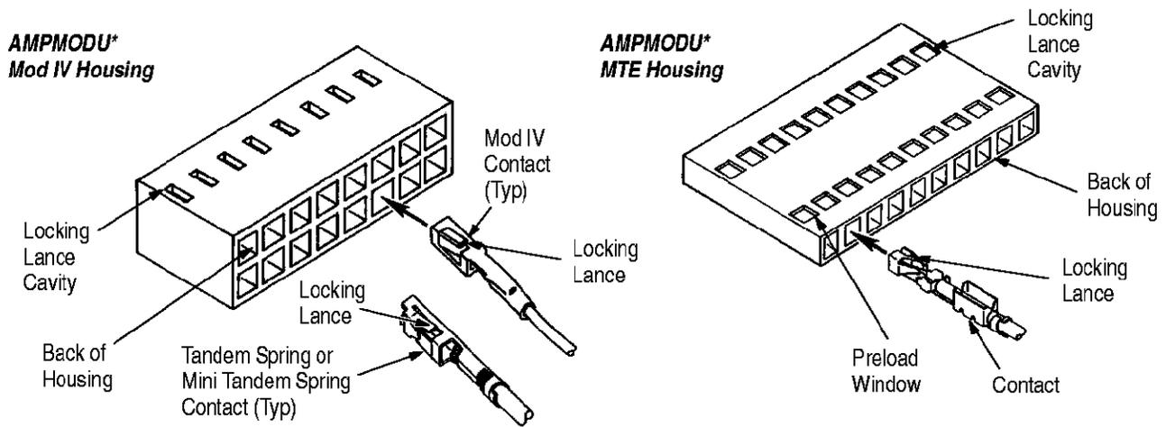
**NOTE:** Contacts shown are typical except that the Mini Tandem Spring contacts are used with Mini Tandem Spring housings only. Also, Mini Tandem Spring contacts are oriented as shown in Figure 3, View B, before insertion into the housing. Refer to Catalog 65816 for Mod IV, Tandem Spring contacts and mini Tandem Spring contacts.
