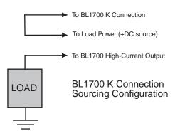
Figure D-7. BL1700 K Connections (Sourcing Configuration)
