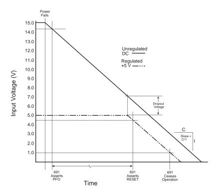
Figure G-2. Power Failure Sequence
