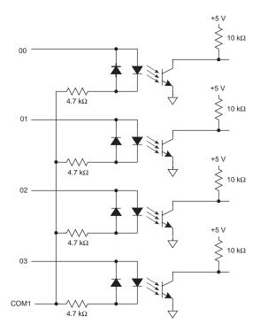
Figure C-8. FWT-Opto Optical Isolation Circuit
