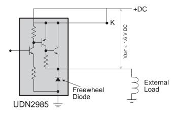
Figure D-3. Sourcing Driver Output
