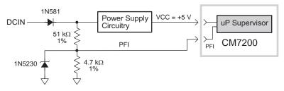
Figure G-1. BL1700 Power-Failure Detection Circuit
