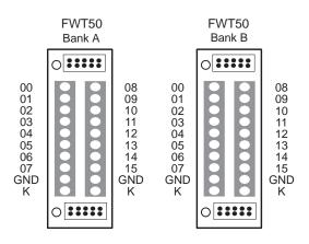
Figure C-5. FWT50 Pinouts
