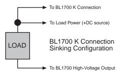
Figure D-6. BL1700 K Connections (Sinking Configuration)
