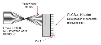
Figure E-2. OP6000 Connection to PLCBus Port
