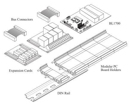
Figure C-11. Mounting BL1700 on DIN Rail
