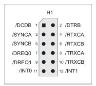
Figure G-3. Pinouts for Optional Header H1
