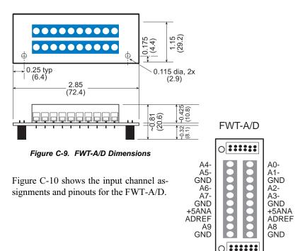
Figure C-10. FWT-A/D Pinouts
