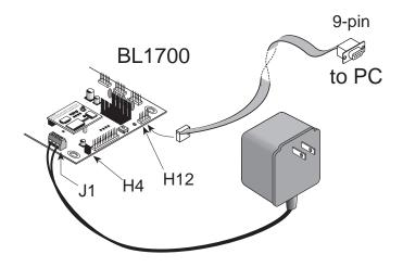
Figure 2-1. BL1700 Programming Connections
