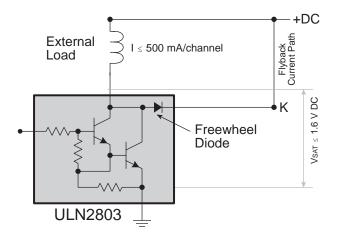
Figure D-1. Sinking Driver Output
