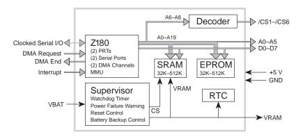
Figure 3-3. CM7200 Block Diagram
