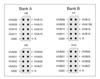
Figure 3-5. Pinouts for BL1700 Digital Input External Connections
