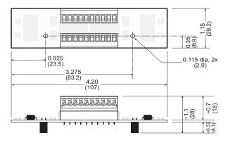
Figure C-6 provides the dimensions for the FWT-Opto module.
