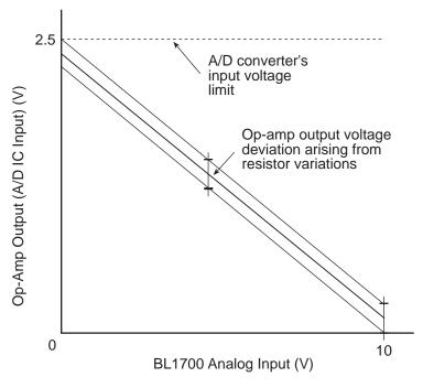
Figure 3-9. Proper Input Range
