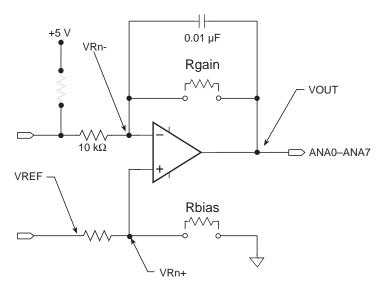
Figure 3-10. Signal Conditioning Test Points
