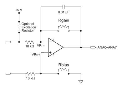
Figure 3-7. Analog Conditioning Circuit
