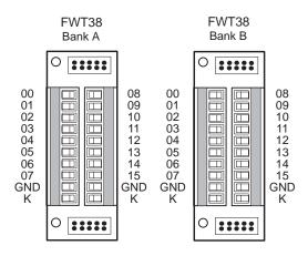
Figure C-3. FWT38 Pinouts
