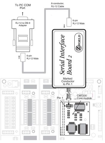
Figure 2-2. SIB2 Connection (BL1700 Top View)
