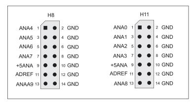
Figure 3-11. Pinouts for BL1700 Analog Input Headers H8 and H11
