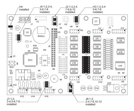
Figure B-2. BL1700 Headers and Factory Default Jumper Configurations
