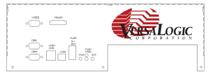
Figure 4. VL-ENCL-5D Front Panel
