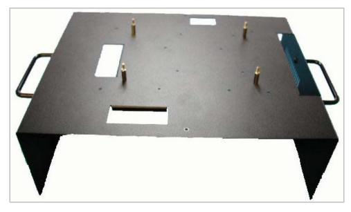
Figure 8. Standoff Positions for EPIC Boards
