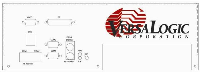
Figure 3. VL-ENCL-5C Front Panel
