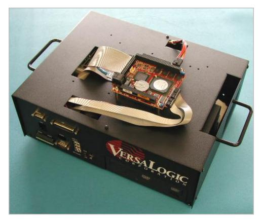
Figure 9. Example PC/104 Board Installation
