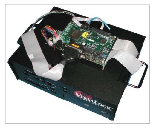
Figure 11. Example EPIC Board Installation
