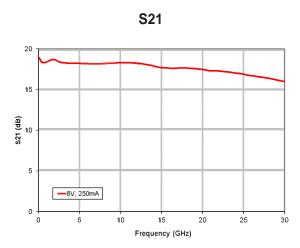
Typical IC performance measured on-wafer
