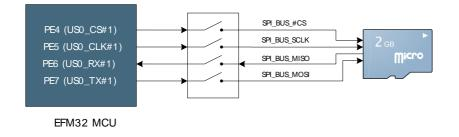
The microSD card slot can be connected to the EFM32 with the BSP function:
