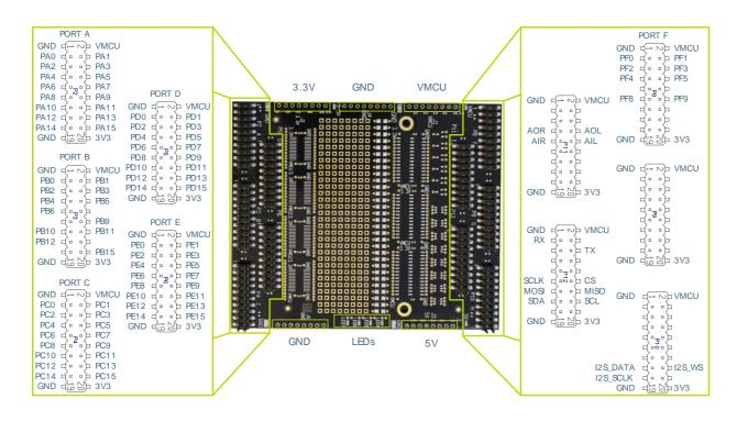
Additionally, the Prototyping Board also contains connection points for different voltages: 3.3V, 5V, GND, and VMCU. Any current drawn from the VMCU pins will also be measurable with the Advanced Energy Monitor, allowing the whole circuit to be evaluated.
