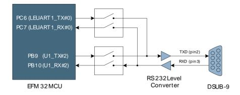
The RS232 peripheral can be connected either to a standard UART peripheral, or to the Low Energy UART (LEUART) of the EFM32.
