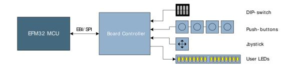
The buttons and LEDs are not directly connected to the MCU, instead the board controller is used to read button states and set the LED outputs. This can be done with a set of BSP API functions
