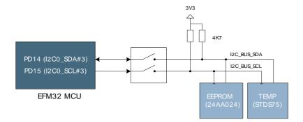
The EEPROM device consists of 256 bytes (256 x 8) and has a lifetime of 1,000,000 erase/write cycles. The EEPROM's  $I^{2}C$  address is 0xA0.
