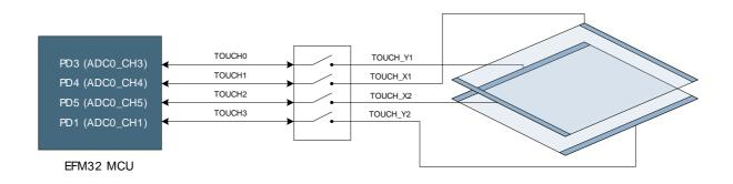
Figure shows how the resistive touch film is connected. When touched, the X-position can be read out by applying a voltage between the X1 and X2 electrodes and measuring the voltage on the Y1 or Y2 electrodes. Likewise, the Y-position can be read out by applying a voltage accross the Y1 and Y2 electrodes and measuring the X1 or X2 electrodes.
