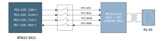
The Ethernet controller has 12KB buffer memory on the receive queue and 6KB on the transmit queue, and supports Auto-MDIX. Two LEDs are placed next to the RJ-45 connector to indicate link speed and activity.
