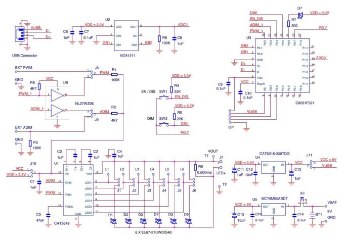
Figure 3. CAT3649AGEVB Board Schematic
