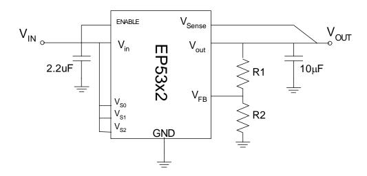
Figure 2. External divider schematic.
