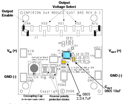
Figure 1. Evaluation Board Layout.
