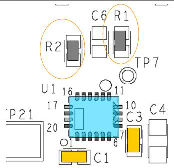
Figure 3. Placement of external divider resistors
