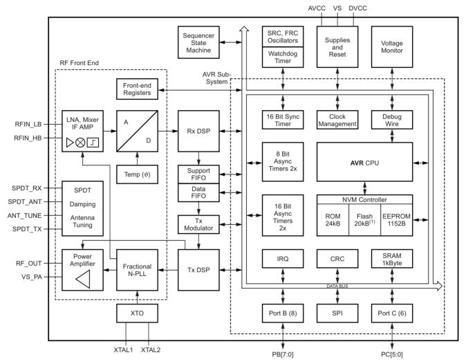
(1) 20kByte Flash for Atmel ATA5831, 20kByte user ROM for Atmel ATA5832, no user memory for Atmel ATA5833
