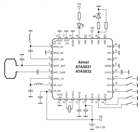
Figure 1-4 shows a stand-alone key fob application circuit for 315MHz or 433.92MHz running from a 3V lithium cell. The Atmel ATA5831/2 stays in OFFMode until one of the NPWRON ports PC1..PC5 is pulled to ground level, waking up the circuit. The NPWRON ports PC1..PC5 have internal  $50k\Omega$  pull-up resistors and can be left open if not used.
