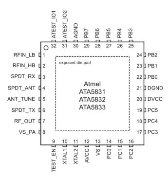
Note: The exposed die pad is connected to the internal die.
