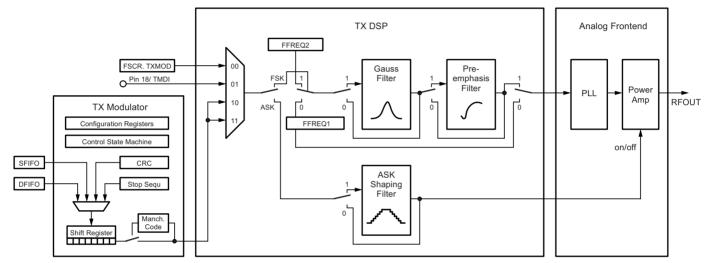
The transmission data source can be selected from a register bit, the transparent input pin 18 (TMDI), and the Tx modulator that fetches the data from the DFIFO and SFIFO.
