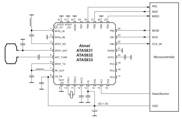
Figure 1-3 shows a key fob application circuit with an external host microcontroller for the 315MHz or 433.92MHz band running from a 3V lithium cell. The Atmel<sup>®</sup> ATA5831/2/3 stays in OFFMode until NPWRON1 (PC1) is used to wake it up. In OFFMode the Atmel ATA5831/2/3 draws typically less than 5nA (600nA maximum at 3.6V/85°C).
