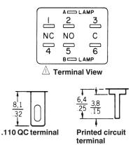
Quick-connect terminals are .110" (2,8 mm) wide by .020" (0,5 mm) thick. The slot is .130" (3,3 mm) long by .048" (1,2 mm). Printed circuit terminals are: Lamp — .025 (0,6 mm) by .020" (0,5 mm): Switch — .025" (0,6 mm) square.
