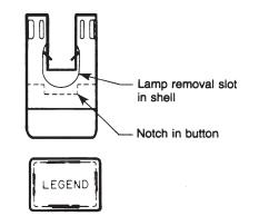
Note: legended button should be assembled as shown above, with button notch keyed to lamp removal slot in shell. This will reduce possibility of lamp droppage when button is removed from the housing. Buttons are legended in this manner.
