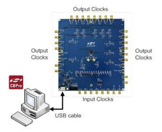
Figure 6. EVB Connection Diagram
