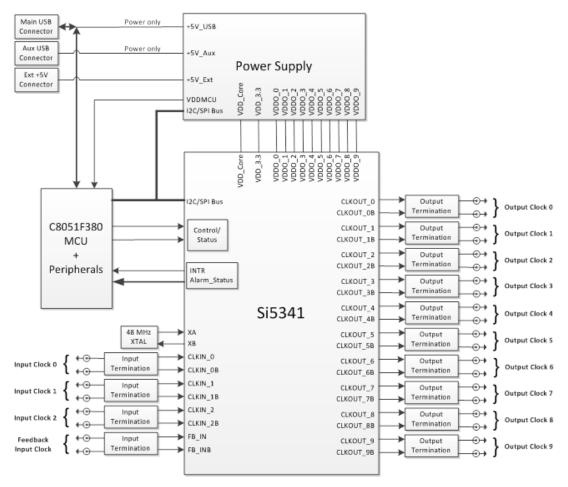
Figure 2. Si5341-EVB Functional Block Diagram
