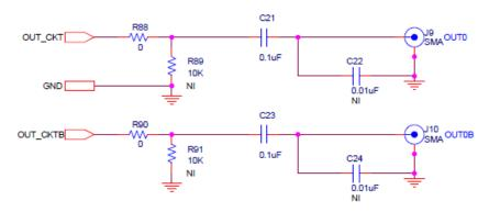
**Figure 5. Output Clock Termination Circuit**
