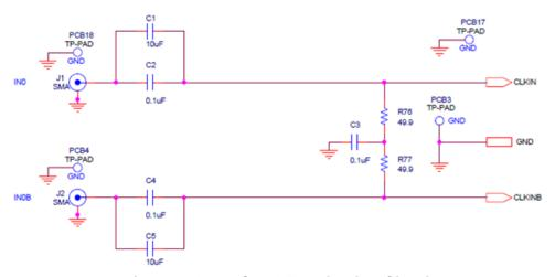
Figure 4. Input Clock Termination Circuit
