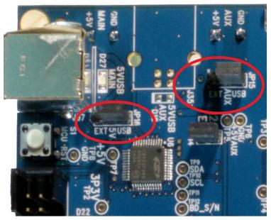
Figure 7. JP15-JP16 Standard Jumper Shunt Installation
