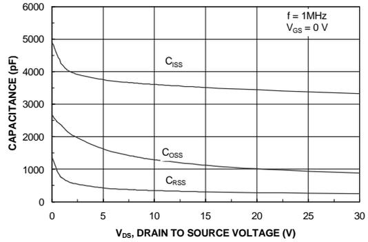
Figure 8. Capacitance Characteristics.
