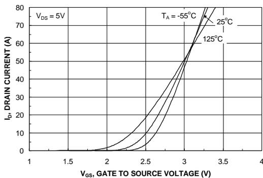
Figure 5. Transfer Characteristics.
