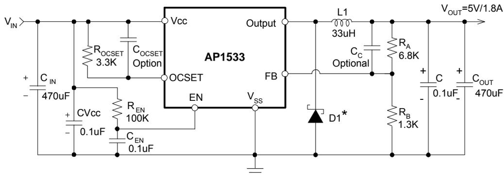
$$V_{OUT} = V_{FB} \times (1 + R_A/R_B)$$
