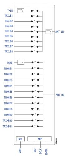
Figure 1. SKY13535-11 Functional Block Diagram
