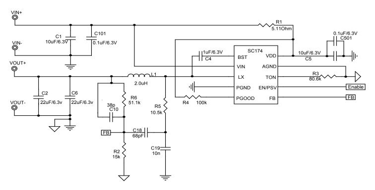
Application Circuit: Buck Converter with 3.3V out and 0 to 4A load current (Vin=5V)
