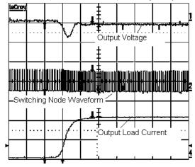
Load Transient Test (V<sub>IN</sub>=5V, V<sub>OUT</sub>=1.2V, I<sub>OUT</sub>= 4A to 0A, Forced Continuous Conduction Mode, L<sub>OUT</sub>=1.3µH, C<sub>OUT</sub>=3x22µF, Channel 1: 50mV/Div, Channel 2:5V/Div,Channel 4: 2A/Div, Time:10µs/Div)
