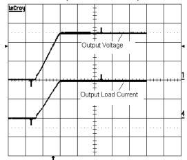
Load Transient Test (V<sub>IN</sub>=5V, V<sub>OUT</sub>=1.2V, I<sub>OUT</sub>= 0A to 4A, Forced Continuous Conduction Mode, L<sub>OUT</sub>=1.3μH, C<sub>OUT</sub>=3x22μF, Channel 1: 50mV/Div, Channel 2:5V/Div,Channel 4: 2A/Div, Time:10μs/Div)
