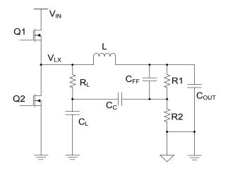
Figure 9 — Signal Injection Circuit
