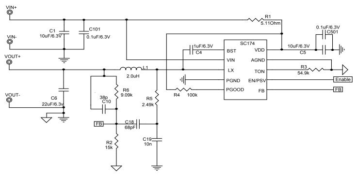
Application Circuit: Buck Converter with 1.2V out and 0 to 4A load current (Vin=5V)
