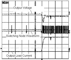
Load Transient Test ( $V_{IN}$ =5V,  $V_{OUT}$ =1.2V,  $I_{OUT}$ = 4A to 0A, PSAVE Mode Enabled,  $L_{OUT}$ =1.3 $\mu$ H,  $C_{OUT}$ =3x22 $\mu$ F, Channel 1: 50mV/Div,Channel 2:5V/Div,Channel 4:2A/Div, Time:20 $\mu$ s/Div)
