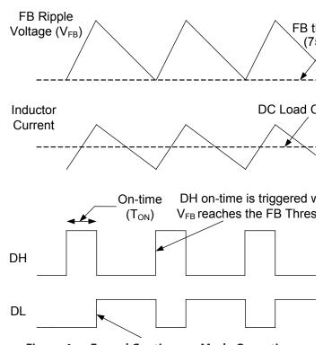
Figure 4 — Forced Continuous Mode Operation
