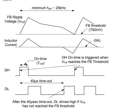
Figure 5 — Ultrasonic Power Save Operation
