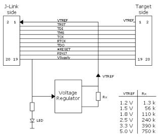
Block diagram of the J-Link Supply Adapter
