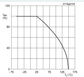
Fig. 2. Normalized continuous drain current as a function of junction temperature
