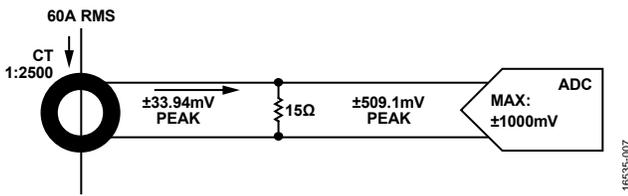
Figure 6. Application Circuit with a Current Transformer Current Sensor on Current Channel B
