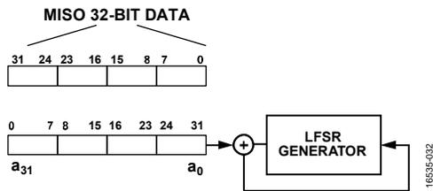
Figure 33. CRC Calculation of 32-Bit SPI Data
