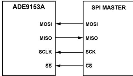
Figure 28. Connecting the ADE9153A Slave SPI Port to a Master SPI Device
