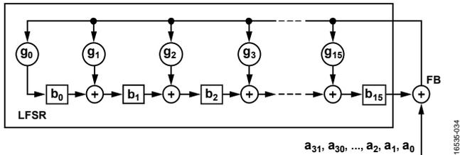
Figure 35. LFSR Generator Used for CRC\_SPI Calculation
