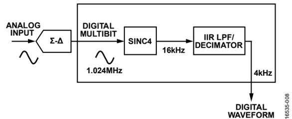
Figure 8. Datapath Following the ADC Stage
