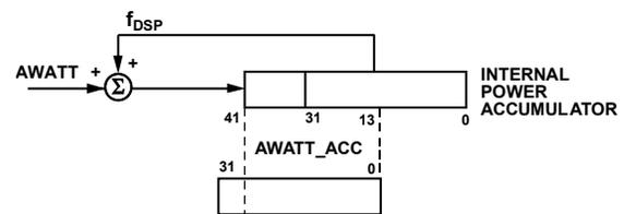
Figure 20. Internal Power Register to AWATT\_ACC
