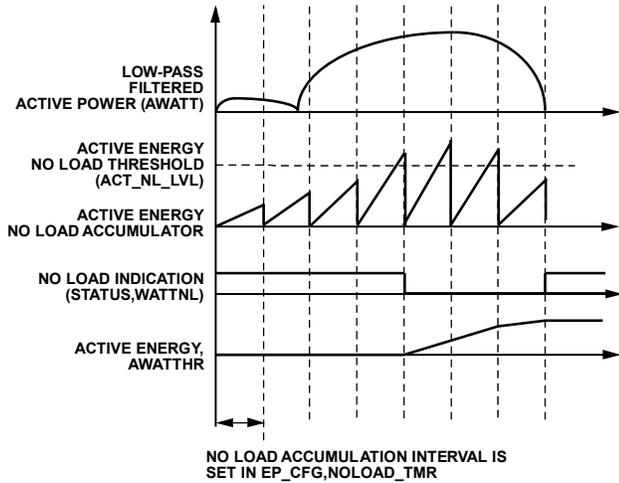
Figure 17. No Load Detection and Indication
