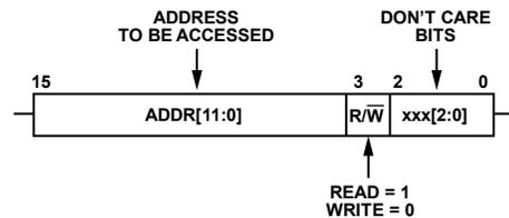
Figure 31. Command Header, CMD\_HDR [15:0]
