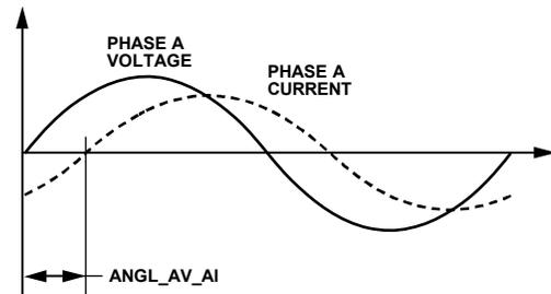
Figure 25. Voltage to Current Phase Angles
