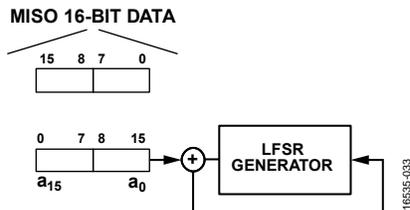
Figure 34. CRC Calculation of 16-Bit SPI Data
