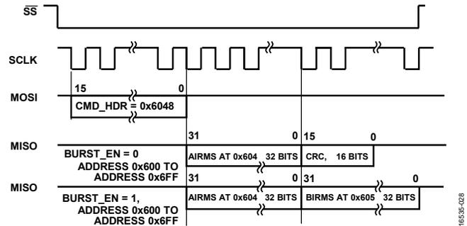
Figure 29. SPI Read Protocol Example—CRC or Next Data Can Follow
