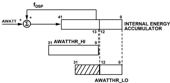
Figure 19. Internal Energy Register to AWATTHR\_HI and AWATTHR\_LO
