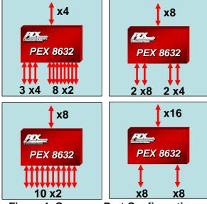
**Figure 1. Common Port Configurations**
