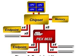
Figure 3. Fan-in/out Usage
