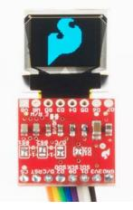
The Micro OLED Breakout Board breaks out a small monochrome, blue-onblack OLED. It's 64 pixels wide and 48 pixels tall, measuring 0.66" across. It's micro, but it still packs a punch – the OLED display is crisp, and you can fit a deceivingly large amount of graphics on there. Most important of all, though, is the Micro OLED is easy to control over either an SPI or I<sup>2</sup>C interface.
