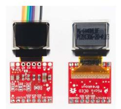
Solder on either side of the PCB. If you're using wire (left) either configuration will do. If you're using headers, we recommend soldering as shown above to the right.
