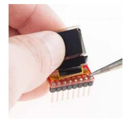
Carefully solder the pins under the connector, which will help stabilize the display in your breadboard.
